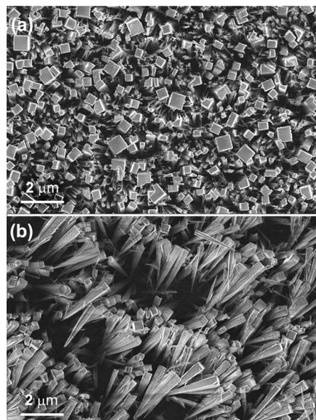
FIG. 3. SEM images of the CVD diamond film surface after oxidation with diamond single crystal pyramids in their original orientation (a) and fallen after gentle touching of the surface by tweezers (b).
