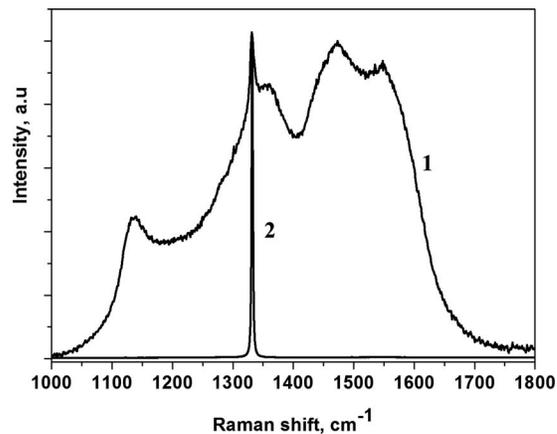
FIG. 2. Typical Raman spectra for as-grown CVD film (curve 1) and for the same film after oxidation (curve 2). The spectra are normalized to the intensity of the Raman line centered at about 1332  $\text{cm}^{-1}$  corresponding to diamond.
