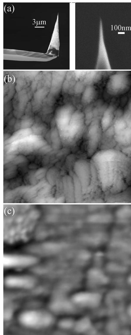
FIG. 4. SEM image of an AFM probe made by gluing a single crystal diamond tip to a silicon cantilever (a). AFM images obtained for the TiN film sample using the diamond probe (b) and the common silicon probe (c). The size of the AFM scans is  $300 \times 300$  nm<sup>2</sup>.
