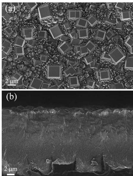
FIG. 1. SEM images of the surface (a) and a cross-section (b) of the CVD diamond film grown under conditions providing rectangular (100) facets on the film surface.
